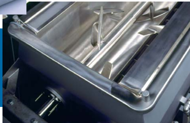
Diverters used with bottom CO 2 injection system. Raised position for sanitation (inset photo).
