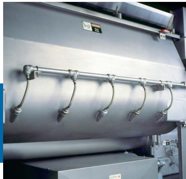
Chilling Systems available with bottom CO 2 injection. Other chilling systems available.
